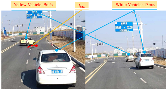
Fig. 12. Lane changing scenario when sensor failure or communication loss.
