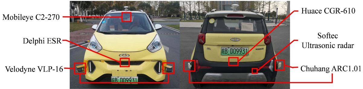
Fig. 2. Sensor deployment of Zhihong intelligent vehicle.
