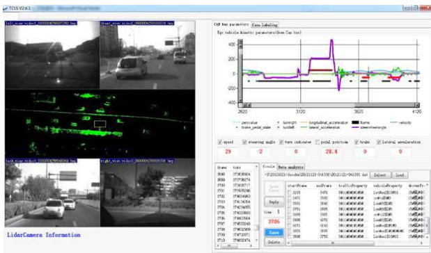
Fig. 6. Labeling GUI. The left area displays the real time LIDAR map and images of the surrounding traffic environment. The top-right area shows the CAN data curves.
